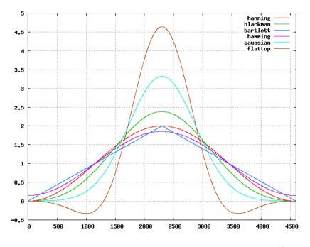
Figure 17.1: Spec and FFT window functions (Gaussian order = 4)
