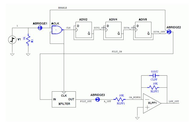
Figure 27.1: Example Circuit C3
