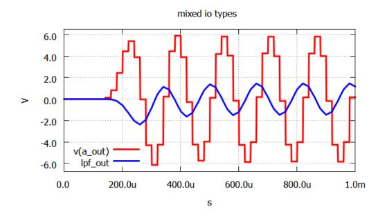
Figure 27.2: Plot of Filter Input and Output
