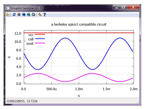
Figure 21.3: VCC, Collector and Emitter Voltages
