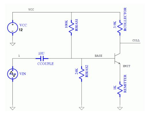
Figure 21.1: Transistor Amplifier Simulation Example
