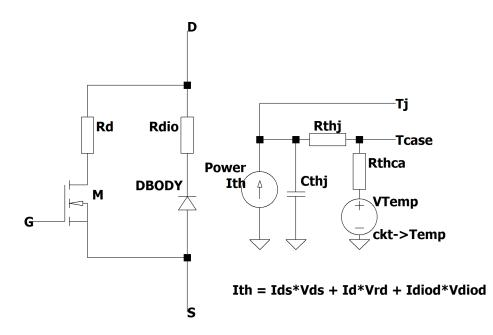
Figure 11.1: VDMOS model including thermal network
