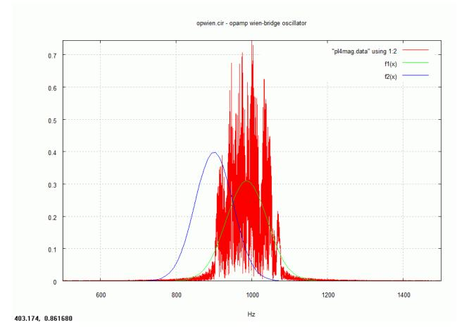
pl4mag.data is the simulation data, f2(x) the starting curve, f1(x) the fitted Gaussian distribution.
