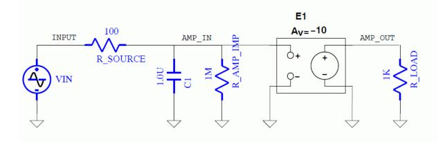
Figure 26.1: Example Circuit 1
