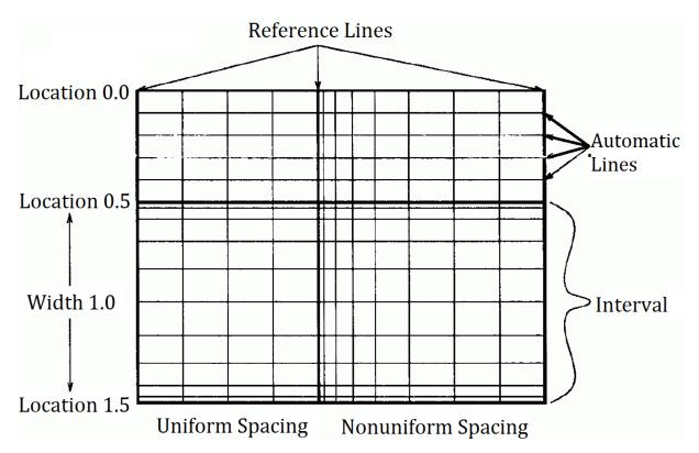
Figure 30.3: Typical mesh for 2D devices
